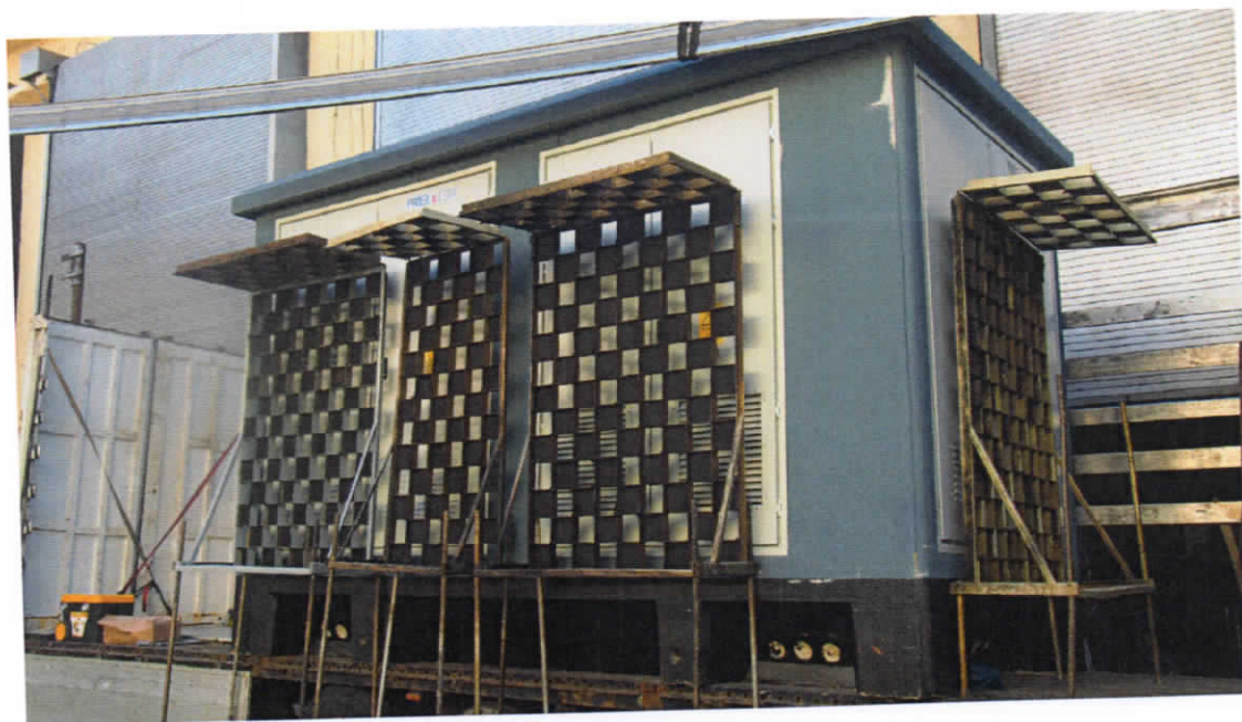
Photos 9 – Aspect of 36/0.4 kV, 1000 kVA Monoblock Concrete Transformer Substation in test circuit after internal arc test for IAC-B
