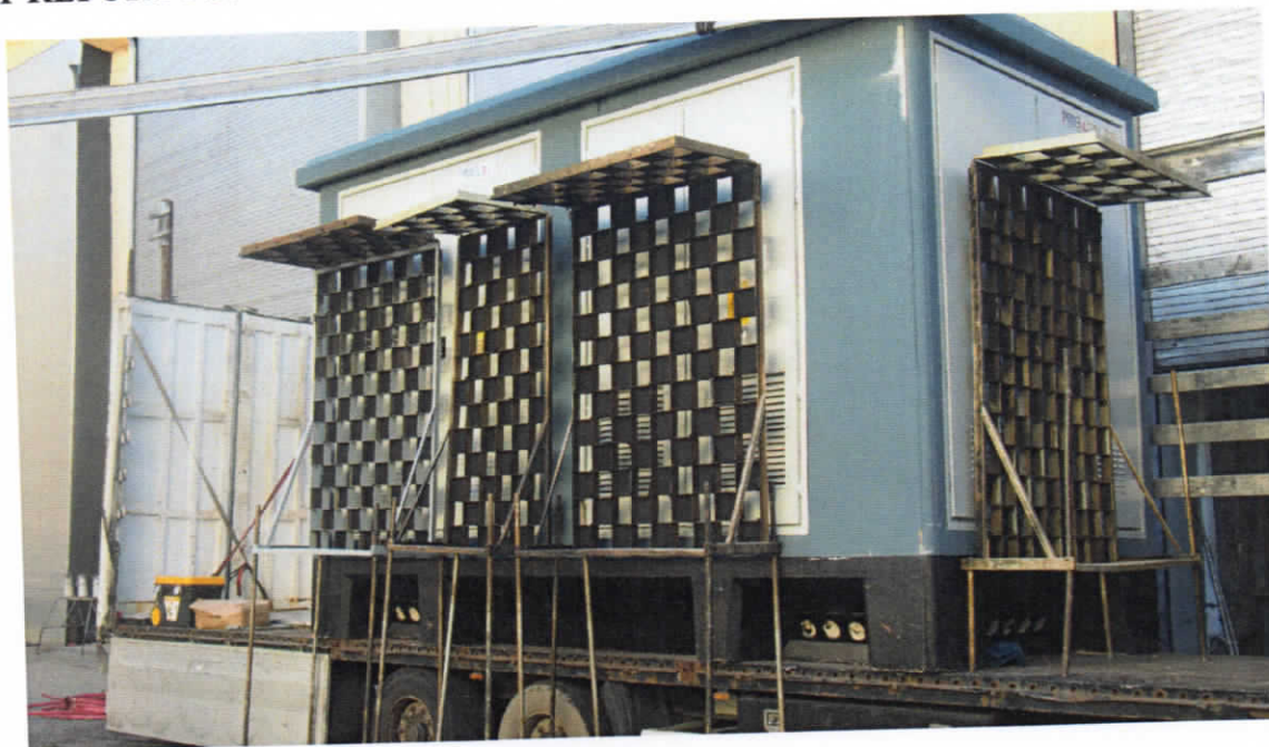
Photo 8 – Aspect of 36/0.4 kV, 1000 kVA Monoblock Concrete Transformer Substation in test circuit before internal arc test for IAC-B
