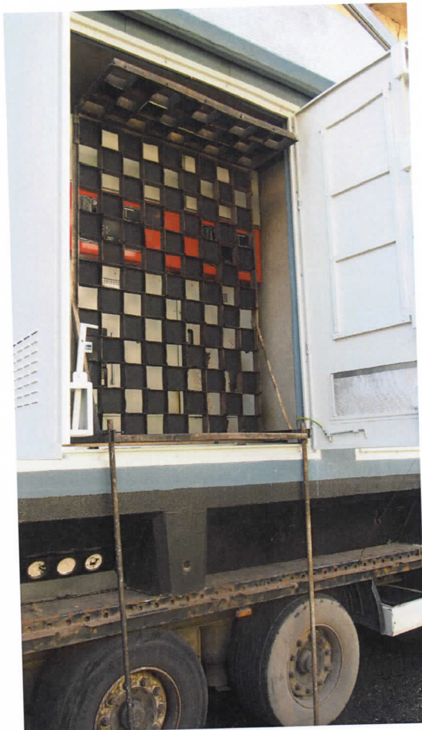
Photo 7 – Aspect of 36/0.4 kV, 1000 kVA Monoblock Concrete Transformer Substation in test circuit after internal arc test for IAC-A
