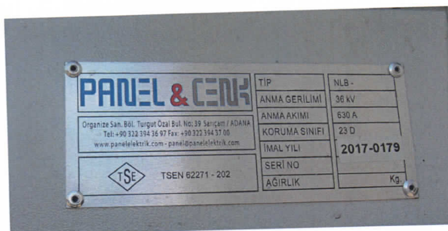
Photos 5,6 – Aspect of 36/0.4 kV, 1000 kVA Monoblock Concrete Transformer Substation with label details in test circuit before internal arc test for IAC-A
